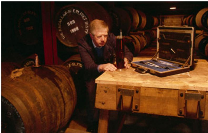
**Alcohol levels** in maturing spirit are regularly checked, and whisky usually diluted prior to bottling – blends typically down to 40% ABV.
